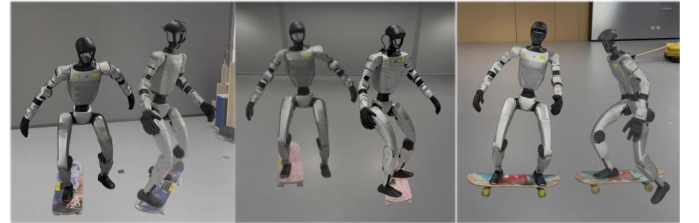
Fig. 12: Humanoid Skateboarding on Diverse Boards. HUSKY enables the humanoid to perform skateboarding behaviors across multiple skateboard platforms, demonstrating the generality and robustness of our method.
